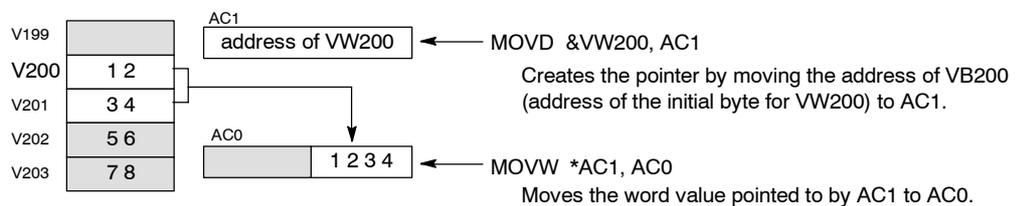
Figure 4-11 Creating and Using a Pointer
