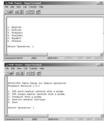
Figure 7-40 HyperTerminal Language Selection and RS-232/PPI Cable Setup
