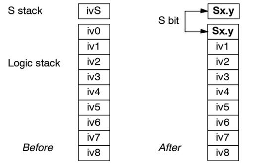
Figure 6-32 Effect of LSCR on the Logic Stack
