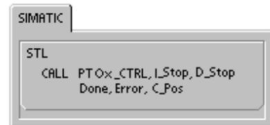
When the Done bit is high, the Error byte reports normal completion with no error or with an error code. See Table 9-7 for definitions of the error codes.
