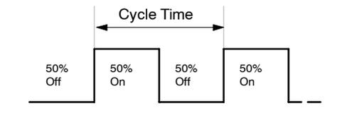
Figure 9-8 Pulse Train Output (PTO)
