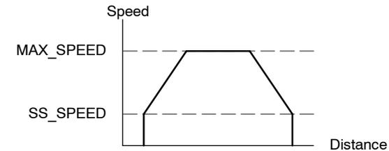
Figure 9-3 Maximum Speed and Start/Stop Speed
