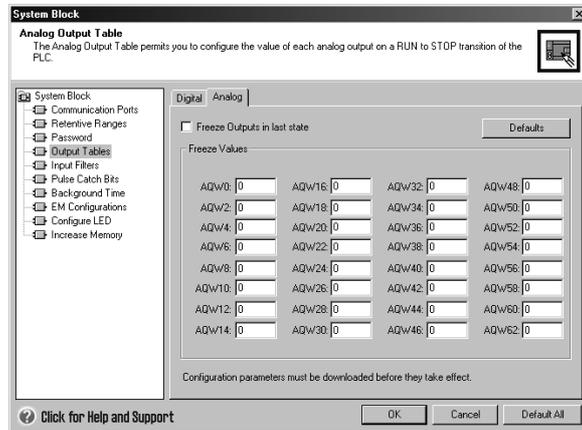
Figure 4-20 Analog Output Table
