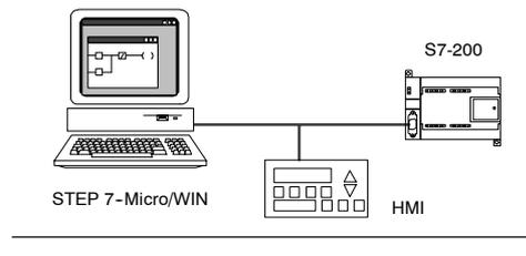
Figure 7-11 Multiple Masters with One Slave
