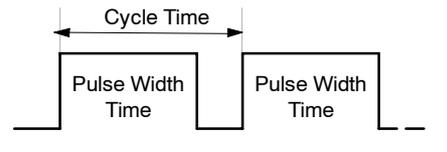
Figure 6-30 Pulse Width Modulation (PWM)
