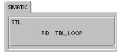
Eight PID instructions can be used in a program. If two or more PID instructions are used with the same loop number (even if they have different table addresses), the PID calculations will interfere with one another and the output will be unpredictable.
