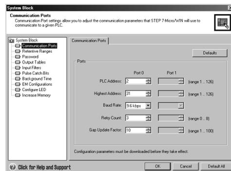
Figure 7-4 Configuring the S7-200 CPU
