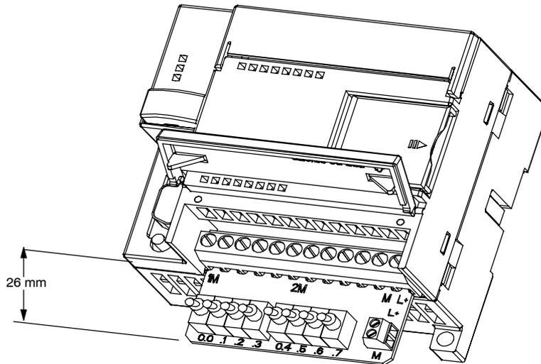
Figure A-43 Installation of the Input Simulator
