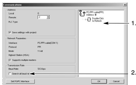
Figure 7-6 Searching for CPUs on a Network
