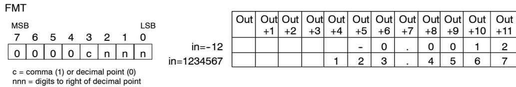
Figure 6-16 FMT Operand for the Double Integer to ASCII (DTA) Instruction
