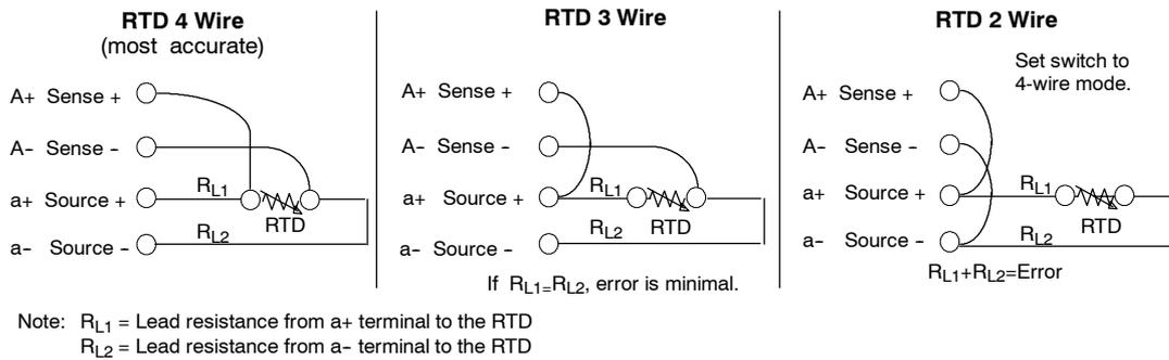
Figure A-22 Wiring the RTD to the Sensor by 4, 3, and 2 Wire
