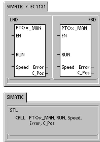
The C\_Pos parameter contains the current position of the module as the number of pulses if the HSC was enabled in the wizard. Otherwise the current position is always 0.
