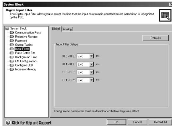
Figure 4-22 Digital Input Filter
