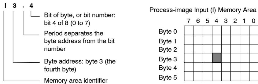
Figure 4-3 Byte.Bit Addressing
