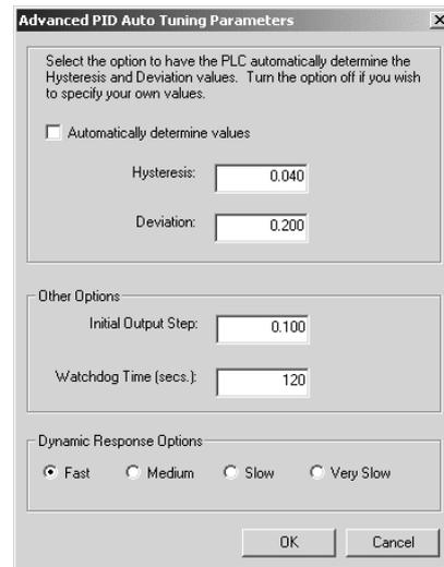
Figure 15-3 Advanced Parameters
