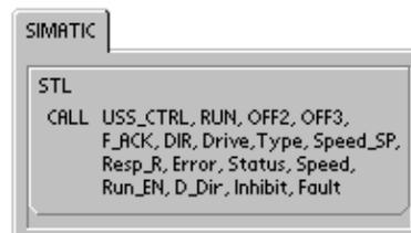
The Drive (drive address) input is the address of the MicroMaster drive to which the USS\_CTRL command is to be sent. Valid addresses: 0 to 31
