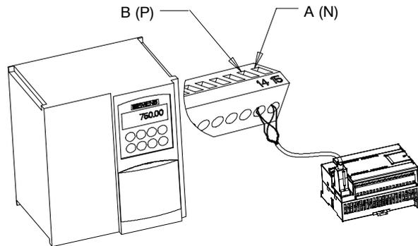
Figure 11-6 Connecting to the MM420 Terminal Block
