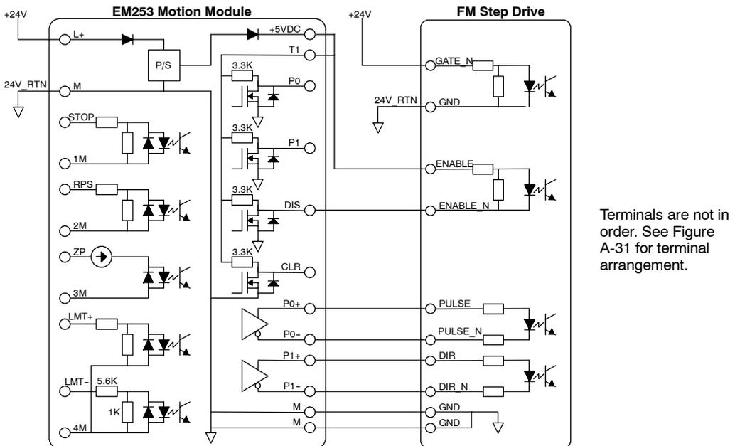
Terminals are not in order. See Figure A-31 for terminal arrangement.
