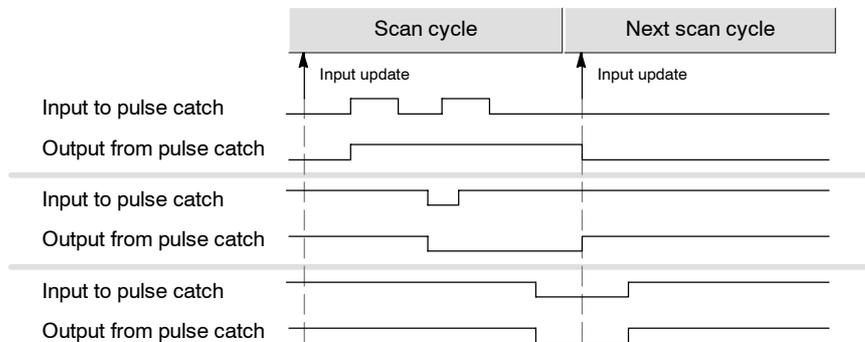
Figure 4-27 Responses of the Pulse Catch Function to Various Input Conditions
