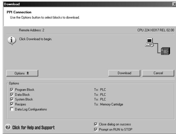
Figure 13-7 Downloading a Project with Recipe Configuration
