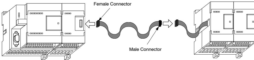
Figure A-40 Typical Installation of the I/O Expansion Cable
