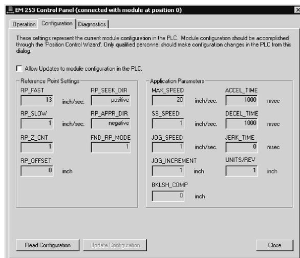
Figure 9-18 Configuration Tab of the EM 253 Control Panel
