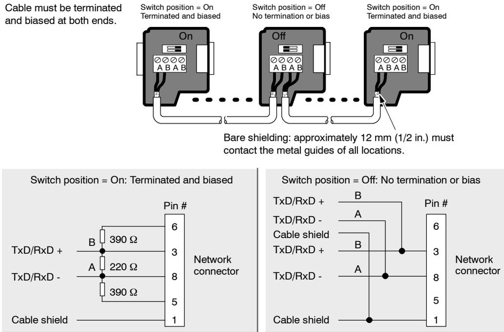
Figure 11-5 Bias and Termination of the Network Cable
