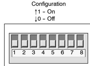
Select RTD type by setting DIP switches 1, 2, 3, 4, and 5 to correspond to the RTD as shown in Table A-30. Refer to Table A-31 for other DIP switch settings.
