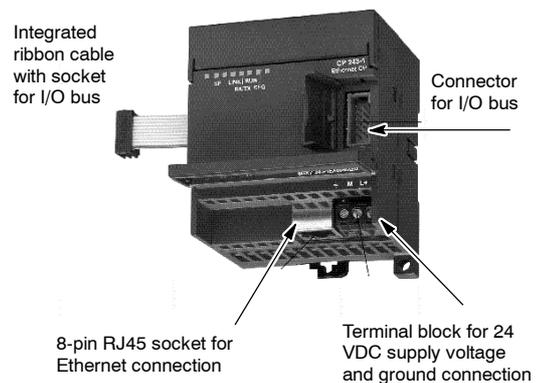
Figure A-37 Connecting the (CP 243-1) Ethernet Module
