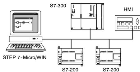
Figure 7-15 Baud Rates Up to 187.5 Kbaud
