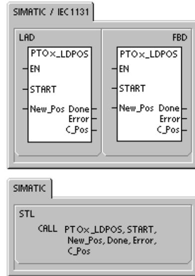
The Done parameter turns on when the module completes this instruction.
